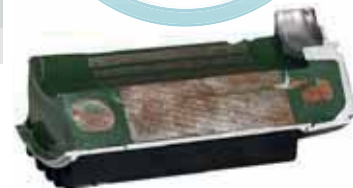
Insulated motor winding cross section
